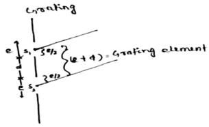
For example if a grating contain 15,000 lines per cm in a grating then the grating element of the grating
